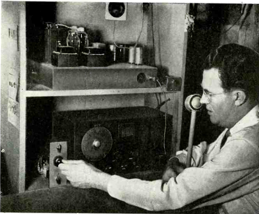
Johnson at the controls of the modified Sky Buddy. A modulator unit is above.
